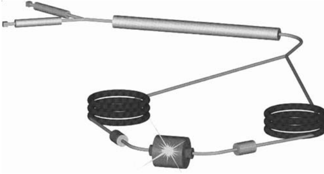
Figure 10.2. Principle of a radiofrequency accelerator for heavy-ion fusion based on the HIDIF study (©Gesellschaft für Schwerionenforschung mbH).
